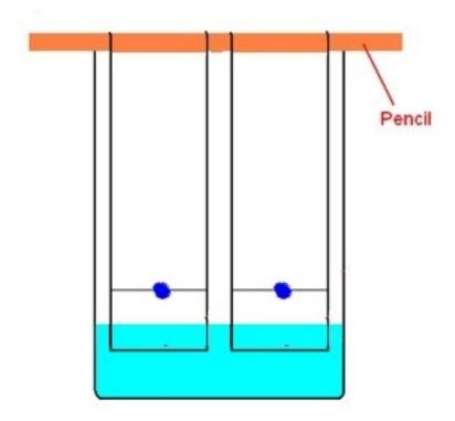
5. Place a pencil across the top of the glass and tape the chromatography paper. Suspend the paper inside the 500 mL beaker.
