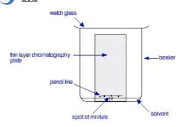
3. As the solvent slowly travels up the plate, the different components of the sample mixture travel at different rates and the mixture is separated into different colored spots.
